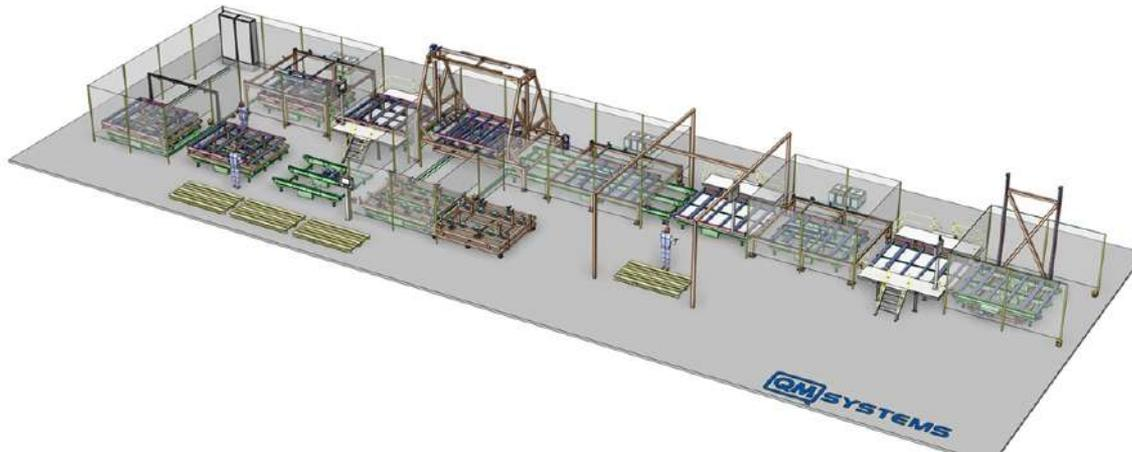
Frame Production Line Overview (Source: QM Systems: Modular Housing Assembly Line, 2020)
