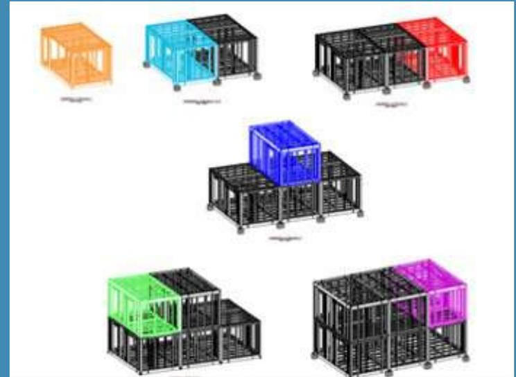
DfMA house built by volumetric method comprising 6 pods
